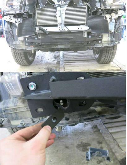
11. Install winch bracket (1) to the chassis using factory bolts, bolts M10x30 (6), nuts M10 (10) and washers (14).
