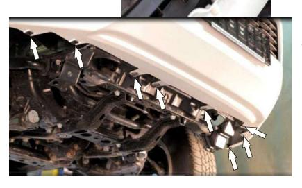
4. Remove lower screws as shown.
