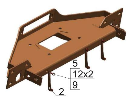
10. Install bumper brackets (2) to winch bracket (1) using bolts M6x20 (5), nuts M6 (9) and washers (12).
