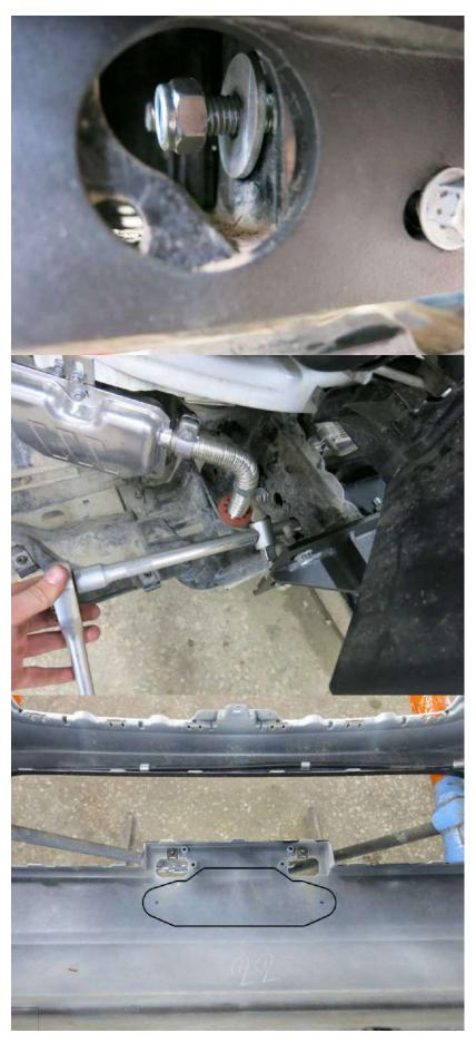
13. Fix winch bracket using bolts M12x30 (7), nuts M12 (11), washers (15 and 17).
