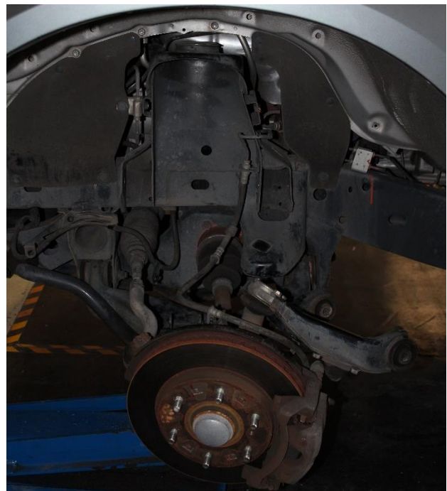
Picture 1: Front Strut Removal
