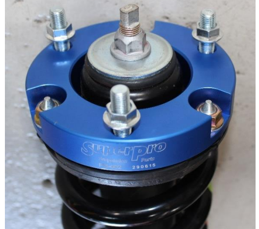
Picture 1: Picture of strut spacer on strut
