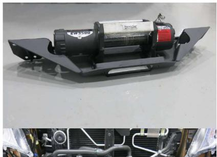
29. Remove the winch bracket from the vehicle, install the winch and pad eye onto the bracket and secure with bolts from the set of winch and pad eye.
