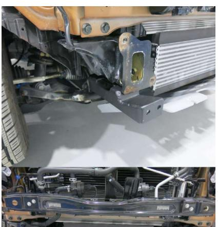
23. Install right frame booster (pos. 3) onto the vehicle frame, secure with standard bolts with installation of standard towing eye. Do not tighten screw joints.
