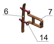
32. Install the number embedded parts (pos. 6 and 7) onto the bumper grille using screws M6x50 (pos. 13).
