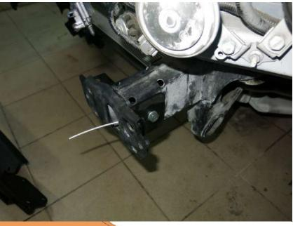
17. From outside of the chassis, mount outer bracket (2) from both left and right side. Fix them with bolts M10x30 (6), washers (8) to insert nuts (5).
