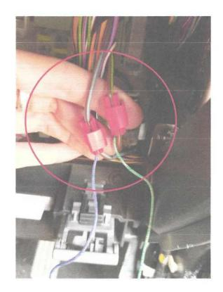
To connect the 12v Power feed, remove the kick plate in the drivers foot well, You find a red permanent live on the connector closest the front of the car, connect to this wire
