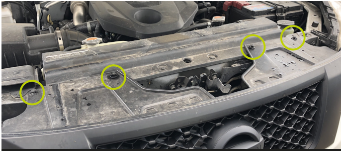
1. Remove trim clips that are located under the bonnet for the front grille.
