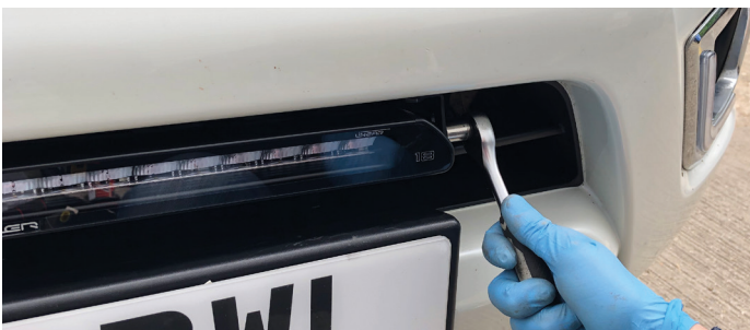
10. Bolt the Linear-18 to the mounting brackets.
