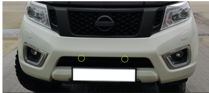
5. Locate the outer upper viens on the lower grille.
