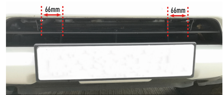
6. Mark 66mm outwards from each vian for pilot hole location.
