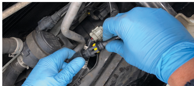
11. Feed lamp cable through to engine bay and plug into wiring harness.
