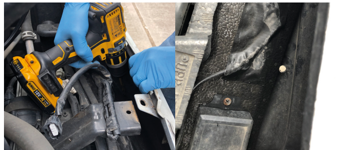
8. Locate the pilot holes from above the grille and drill to 8mm diameter.
