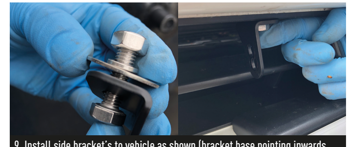
9. Install side bracket's to vehicle as shown (bracket base pointing inwards, straight edge forward).
