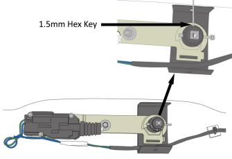
5. Once the grub screw has been removed take the insert from the centre of the barrel and also remove the pin through the centre of the barrel.
