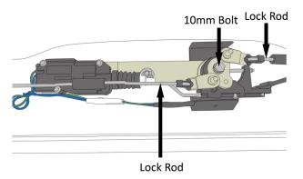
3. Remove the nuts on each end of the actuator rod and take away the rod. Remove the nut on the pin protruding from the lock barrel area on the handle before removing the black housing on the back of the handle.
