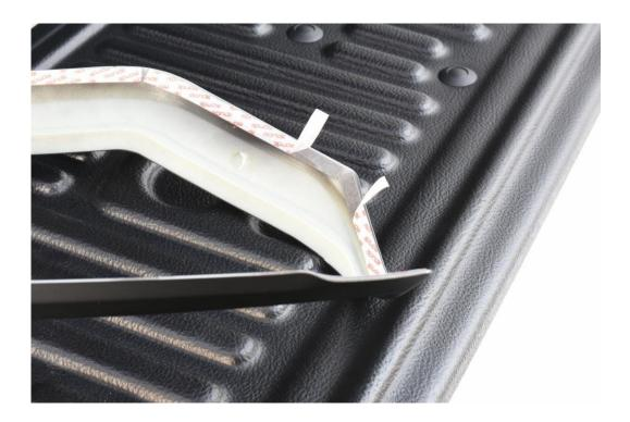
Offer the tail lamp surround into position on the tail lamp of the vehicle leaving the tabs exposed.
