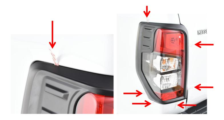
Once happy with the positioning of the tail lamp surround pull each of the tabs to fully expose the adhesive tape on the rear of the surround. Press firmly around the edge of the tail lamp surround to ensure the adhesive has made contact with the tail lamp.
