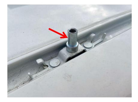
At this point you can choose to reinstall the trim plastic making sure to cut at the points of the four connection bolts. Once trim has been replaced or discarded and making sure each of the feet of the roof rails have a rubber gasket. Place the bars onto the vehicle so the previously fitted connection bolts should now sit inside the roof rails.
