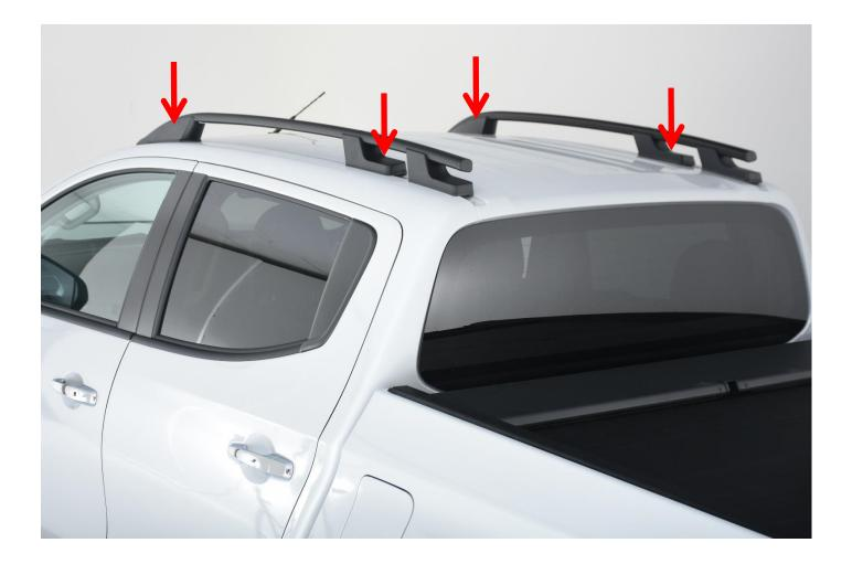
Take the supplied M8x40mm cap screws with an M8 washer and use these to secure the front feet of the roof rails into the connection bolts. Take the M8x50mm cap screws with an M8 washer and secure the middle feet of the roof rails into the connection bolts.
