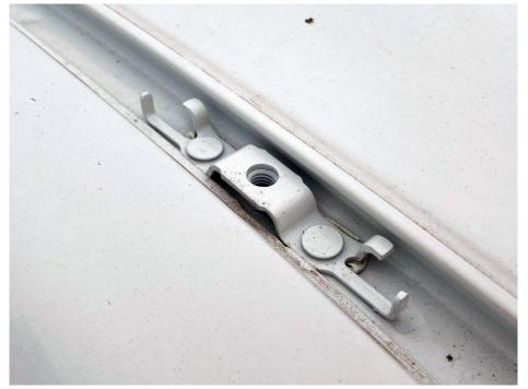
Offer up a roof rail to the vehicle and make note of which two mounting points will be used during the installation of the bars on each side. Take the supplied M8 connection bolts and insert into the noted mounting points on both sides of the vehicle as shown in the image.
