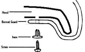
4. Apply the anti-abrasive tape on edge of hood where plastic fastening clip secures the Bonnet Guard near the fenders. Use the supplied alcohol prep-pads to cleanse the area first.
